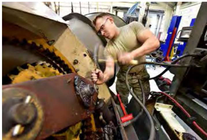
• Tech. Sgt. Jacob Graham, a 173rd Fighter Wing vehicle operations mechanic, removes a cotter pin from a damaged plow roll-over assembly, Jan. 8, 2019 at Kingsley Field in Klamath Falls, Ore. The parts for this older plow are growing harder to find, and the mechanics will have to fabricate one part on-site in order to return this snow plow to service. (U.S. Air National Guard photo by Tech. Sgt. Jefferson Thompson)
